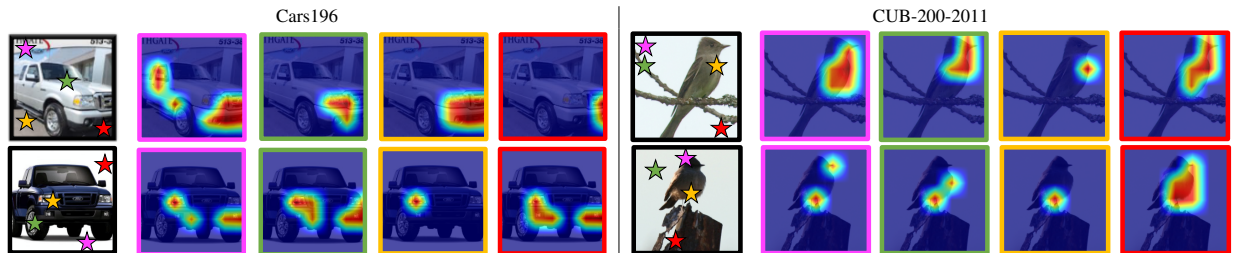
Figure 6. Qualitative examples of SOA maps on the Cars-196 and CUB-200-2011 datasets. (a) corresponds to Cars196 dataset and (b) corresponds to CUB-200-2011 dataset. Each row depicts the source image and four corresponding SOA maps obtained for specific spatial locations (marked by stars).
